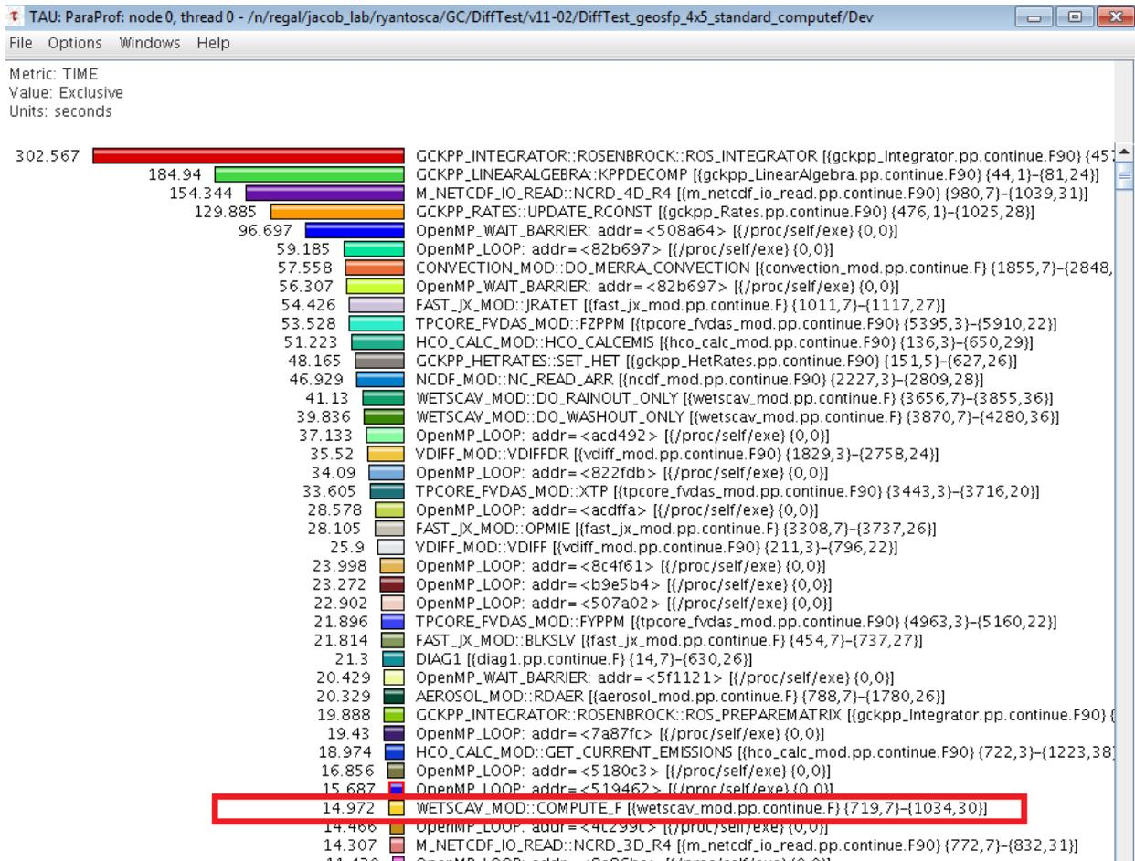
After parallelizing the loop, the COMPUTE\_F routine now only spends 14 seconds on the master CPU, instead of ~400 seconds. This means that the work of calling COMPUTE\_F is now being efficiently split up among all 8 CPUs. This should result in a significant speedup.
