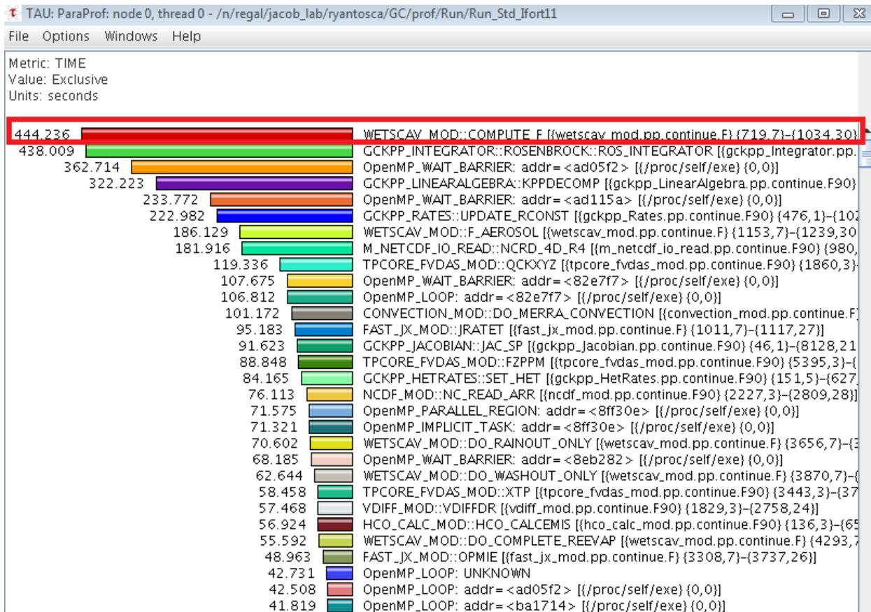
As you can see, because the COMPUTE\_F routine was not being called from a parallel loop, the subroutine was only being executed on the master CPU. This caused a slowdown because the other CPUs were being forced to wait until COMPUTE\_F finished before the simulation could proceed.
